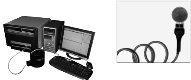
Fig. 2 The diagram of the Hot Disk TM thermal constant analyzer and sensor.
